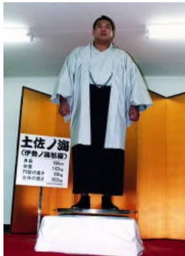
Figure 4 The standing Japanese Sumo (wrestling) wrestler weighing 142 Kg on the magnet weighing 60 Kg is levigated by superconductor placed below the white cloth whose magnetic susceptibility as diamagnetic material is strongest ( $\chi_m = -1$ ). The total weight above the superconductor is 202 Kg. This phenomenon was made it possible by so-called the Meissner effect.
