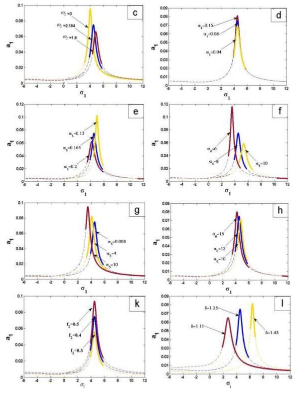
Fig.10 Stability of the practical case (in the second resonance case),  $a_2 \neq 0$  on steady state amplitude  $a_1$  against  $\sigma_1$
