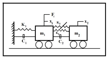
Figure1 Schematic graph of ultrasonic machine
