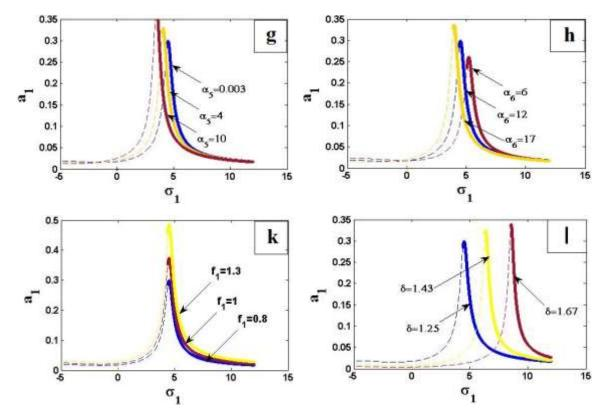
Fig.9 Stability of the practical case (in the first resonance case),  $a_2 \neq 0$  on steady state amplitude  $a_1$  against  $\sigma_1$
