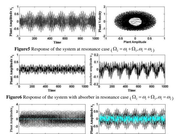
Figure7 Comparison between Responses of the system under effect of absorber in resonance cases
