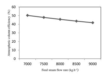
Fig. 7: Effects of changing the flow rate of the feed steam on the exergy efficiency of the atmospheric distillation column
