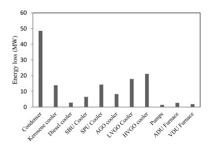
Fig.2: Energy losses in the different components of the CDU
