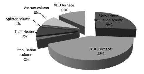
Fig.3. Distribution of exergy losses in the different process components
