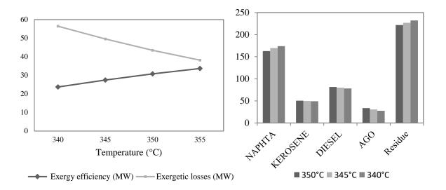
Fig. 8: Effects of changing the furnace outlet temperature on the exergy loss and efficiency of the atmospheric distillation column
