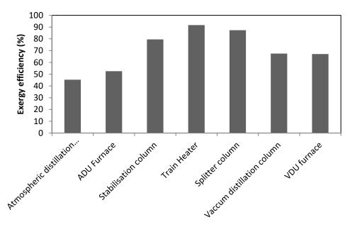
Fig. 4: Exergetic efficiency of the different components of the crude distillation unit
