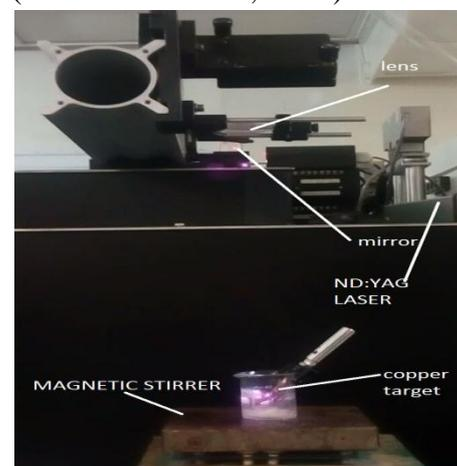
**Fig 1. Experimental Setup of LASIS**
