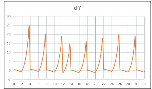
Figure 6. The difference between the precise and broadcast orbits in  $Y_{ECEF}$  direction Horizontal axis is time in hours and vertical axis the difference in ms
