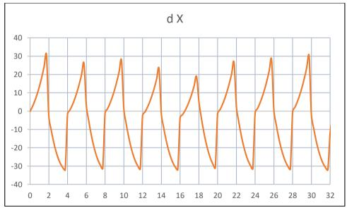
Figure 5. The difference between the precise and broadcast orbits in X<sub>ECEF</sub> direction Horizontal axis is time in hours and vertical axis the difference in ms
