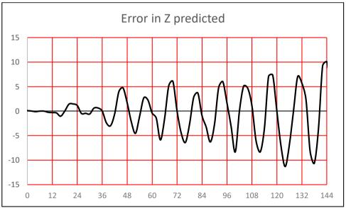
Figure 10. Errors in calculating orbit. Horizontal axis is time in hours and errors in predicted  $Z_{ECEF}$  in ms is y axis
