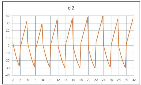
Figure 7. The difference between the precise and broadcast orbits in Z<sub>ECEF</sub> direction Horizontal axis is time in hours and vertical axis the difference in ms
