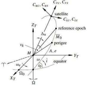
Figure 2 : Keplerian and perturbed parameters in broadcast ephemerides [4]
