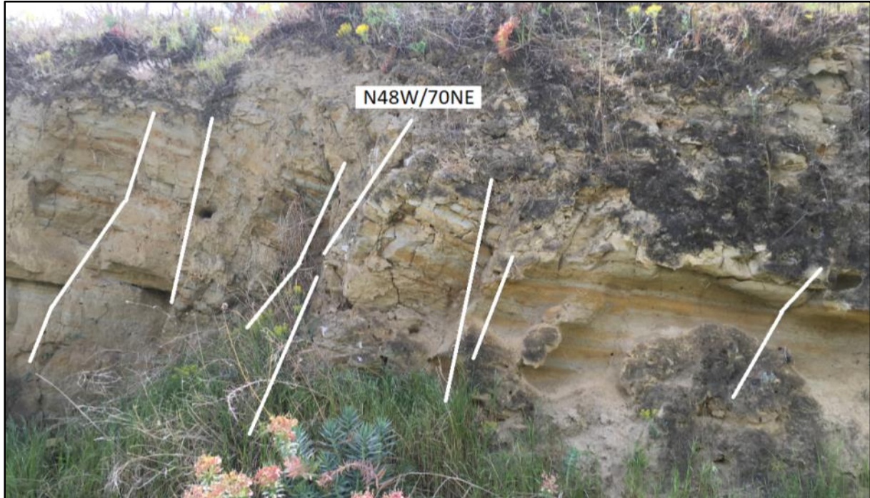
Figure 8. Fractures and fault zone on Kocadetre at west of Celtikci (look to E)
