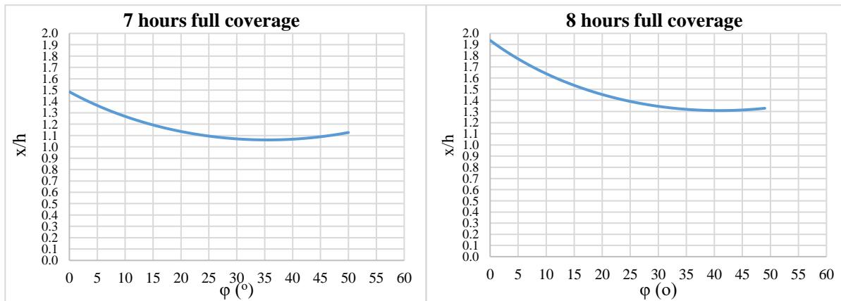
Figure 14. Graphical representation of variation of  $x/h$  ratio on the day of the summer solstice (June 21<sup>st</sup>) for different latitudes and different hours (1 to 8 hours) of full exposure to the direct solar beam of all PV arrays.
