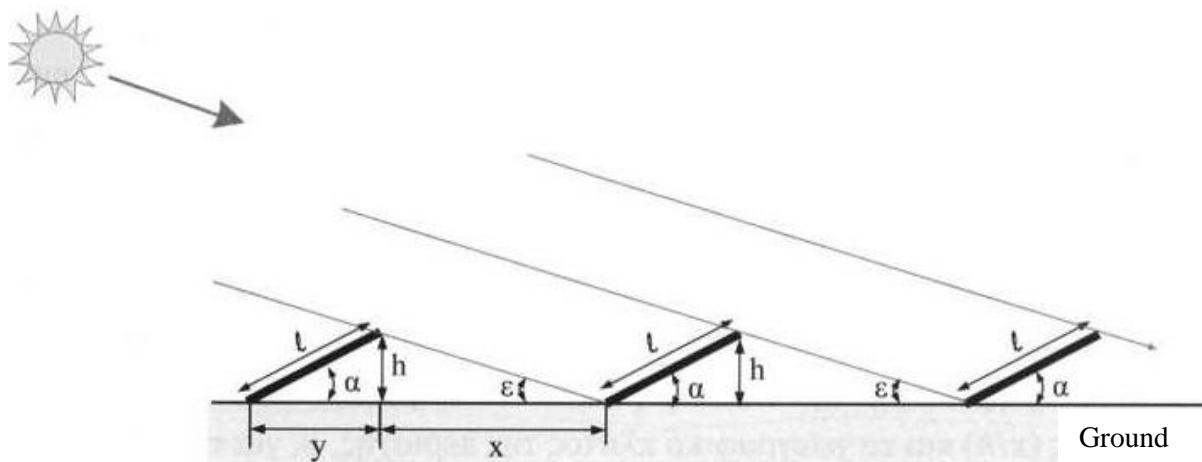
Figure 11. The geometry for the placement of consecutive PV modules of rows, on horizontal ground facing south.
