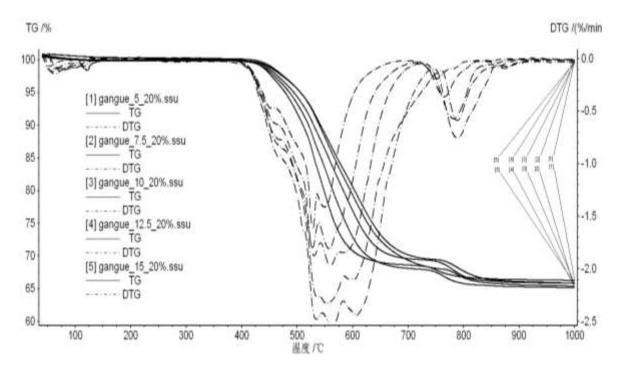
Fig 3.1, 20% O2 concentration TG-DTG curve at different heating rates
