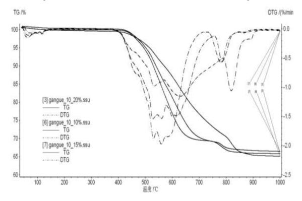
Fig 3.2,10 °C / min heating rate different concentrations of O2 TG-DTG curve
