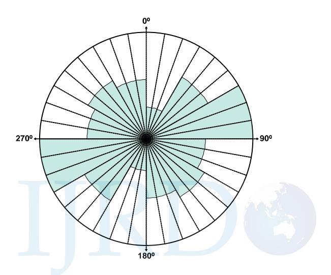
Fig 4. Rose diagram showing the Trends of the Fractures/Joints found within the study Area.
