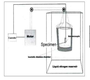
Fig1. Cryogenic treatment system
