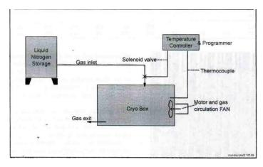
Fig 3. Cryogenic equipment
