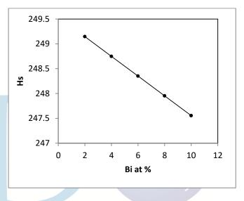
Fig 6: Variation of average heat of atomization per single bond H<sub>s</sub> with Bi content
