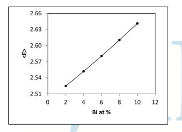
Fig 4: Variation of overall mean bond energy with Bi content
