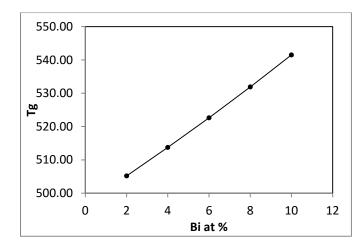
Fig 5: Variation of glass transition temperature  $T_g$  with Bi content
