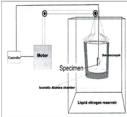
Fig1. Cryogenic treatment system
