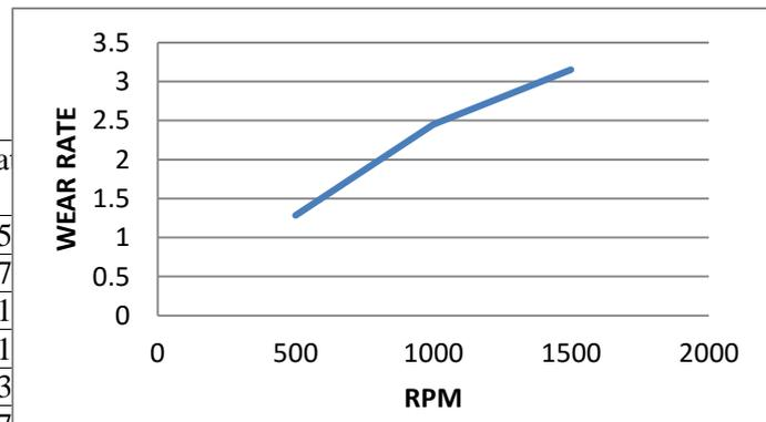
Fig.8 RPM VS WEAR RATE
