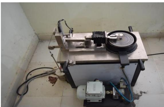
Fig 2. Pin-on-disc wear testing Machine
