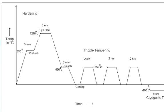
Fig 5. Heat treatmet and cryogenic treatment cycle for AISI T42
