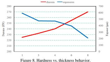
There is an inverse relationship between hardness and thickness, the latter being reduced by the effect of fluid friction on the surface and causing a decrease in grain size due to the effect of pungency.
