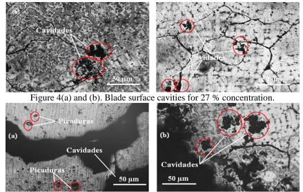
Figure 5(a) and (b). Blade surface cavities for 34% concentrations.
