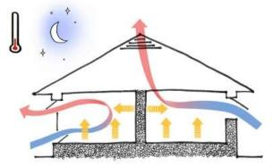
Fig. 6 difference between day and night ventilation
