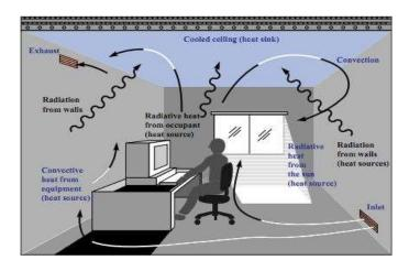
Fig. 1 Explination of radient coolong system in figure.
