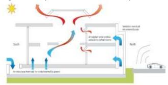
Fig. 2 supplying and removing air through an indoor space by natural means
