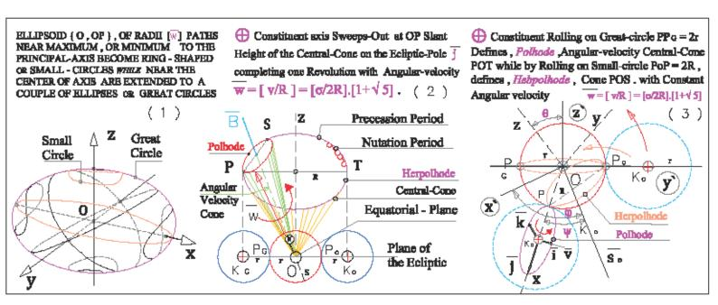
**Figure.20.** In (1), are shown different Paths near maximum or minimum Principal axis from where become-ring shaped or Small-circles while near the center of axis extend to a couple of ellipses or Great-circles .For a constant Angular-velocity ,**w**, and by changing torsional momentum ,**B**, only then Infinite curves are possible for the motion .
