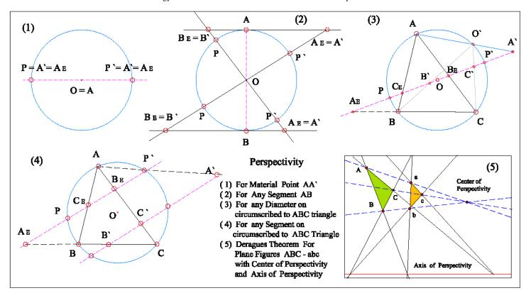
**Figure.3.** Pole and Axis of Perspectivity for Points , Sectors , Planes , Volumes.
