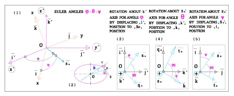
**Figure.17.** In (1) are shown Euler angles {  $\phi$ ,  $\vartheta$ ,  $\psi$  } in a *Fix*-Three-Coordinate-System x , y , z through ,O, and one *Movable* x`, y`, z` at ,O . In (2) is shown the Spearhead ,P , of OP Angular-velocity  $\overline{w}$  vector , and the Tangential Plane ,E ,to Angular-velocity-Ellipsoid  $\overline{w}$  , on Momentum vector  $\overline{OT} = \frac{2L}{R}$
