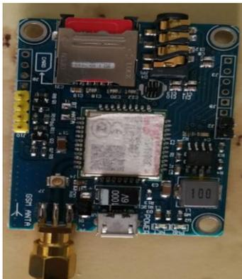
Figure 6. Shows GSM sim800c Modem
