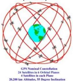
Figure 1. Typical GNSS System with 24 satellites in constellation for global coverage (Source: Mahesh, 2014)
