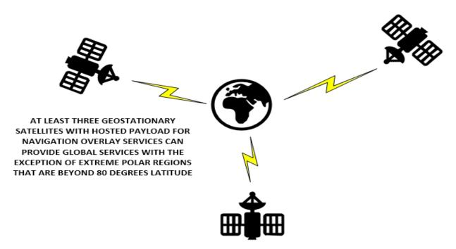
Figure 4: Illustration of use of Geostationary Satellites for Total Global Coverage.
