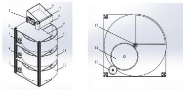
1- Raspberry Pi 3b+; 2-Connecting rod; 3-Servo 1; 4- Servo 2; 5-Servo 3; 6-Detection box; 7-Servo 4; 8-Baffle; 9-Support plate; 10-Storage plate 1; 11-Storage plate 2;12-Turntable 3; 13-Pinion; 14-Large gear; 15-Middle gear.
