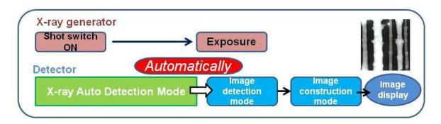
Fig. 4. Pictorial representation of X-ray detection and image display process.
